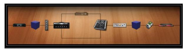
This is a clean patch with Mesa Dual Rectifier(treadplate) were I have the Noise Gate and StudioEQ (to lower the gain) before the amp and after the amp smart harmony followed by a tube compressor and finally delay and reverb. Note that the smart harmony id in path A, so I can mix it with the unaffected signal from path B (see the chapters on "understanding the mixer block" and "amp positioning" for more details on parallel and serial processing)
