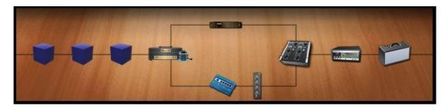
In this example the signal goes to the amp first and then the two paths are processed in parallel and merged in the mixer block.
