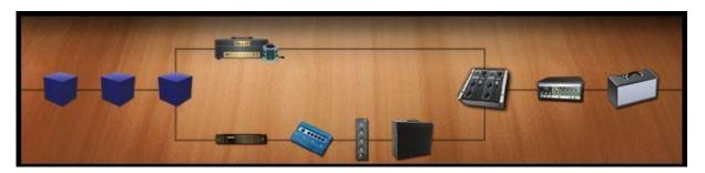
Again, we make use of parallel processing. In path A the signal is processed through the amp and in path B a clean signal is passed through the two effect modules. NOTE: make sure the bypass volume (BYP VOL) is maxed out (100%) if you intend to (de)activate the amp (in path A) with a footswitch and you still want a signal to pass through path A.
