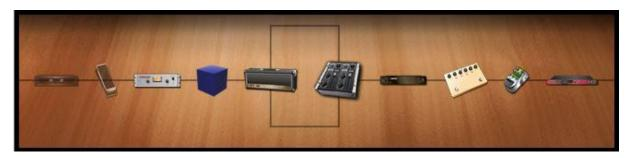
If we move the two effects after the mixer block to patch A and B we will get a parallel signal chain, the effects in these paths are processed simultaneously.
