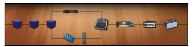
This is basically the opposite first the signal is parallel processed in path A & B before it is merged in the mixer block and send to the amp.
