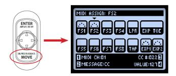
Choose which Footswitch you want to use. Note that in ABCD mode FS5 thru FS8 are used for the ABCD patches.
