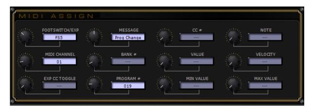
The operation is basically the same, in this example I have set the program change value for patch A (which is FS5) to program 19 on the external preamp.
