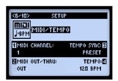
As you can see I use **MIDI channel 1** for exchanging information (you can choose any of the available 16 channels) And secondly I have set the MIDI out/thru to **OUT. Note:** Make sure the receiving device is *listening* to the same MIDI channel!
