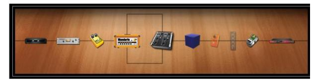
In this example I begin with a noise gate, then compressor and overdrive followed by the amp. After amp I use a phaser and StudioEQ (for volume compensation) and finally a delay and reverb.
